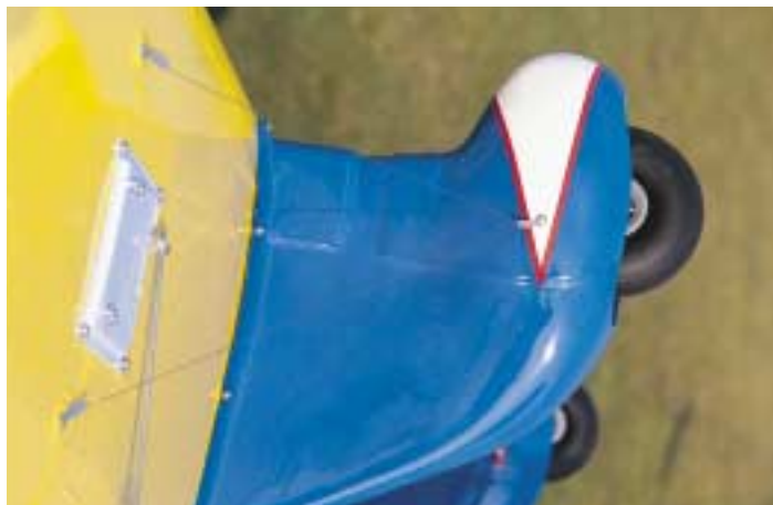
Above: I thought the landing-gear legs were too flexible, so I added an additional support. I secured it to the gear leg and to a hard point that I added to the wing.
