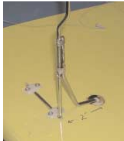
Above: I thought the landing-gear legs were too flexible, so I added an additional support. I secured it to the gear leg and to a hard point that I added to the wing.
