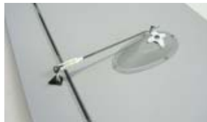
Aileron servos are concealed by plastic covers. Each aileron is driven by a separate servo.
