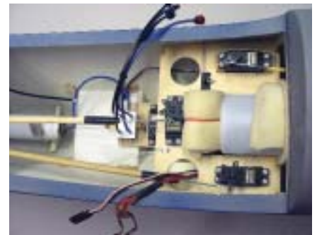
The fuselage interior is spacious; it has ample room for the radio gear, air cylinder and retract valve.
