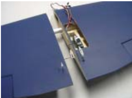
The wing is joined using a tube spar, and an aluminum pin is used to align the two panels. Flaps are driven by a single servo that is connected by a split linkage to the two torque rods.
